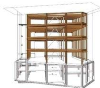
250 YEAR STRUCTURE HEAVY TIMBER, CONCRETE & STEEL
