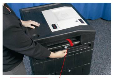
Unlock and open Auxiliary Slot Step 21
