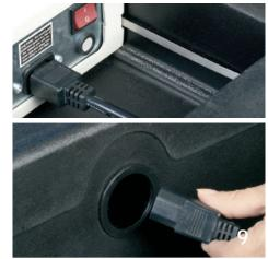
Turn off the AccuVote unit by pressing the red ON/OFF switch on the back of the unit. Unplug the power cord from the UPS unit, unplug the unit and remove the power cord. Repack the unit in its case.
