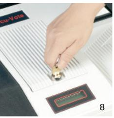
When all copies of the Summary Results Report needed have printed, replace the printer cover and lock the printer using the plain brass key. Slide the AccuVote forward to access the power switch.
