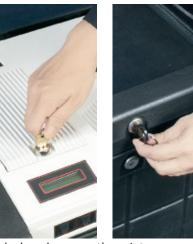
Unlock and remove the printer cover using the plain brass key. Unlock and open the retaining door of the ballot box using the brass key with plastic key cap.
