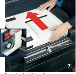
Power the AccuVote unit on by pushing the red ON/OFF switch on the back of the unit and then finish sliding the unit firmly into place.
