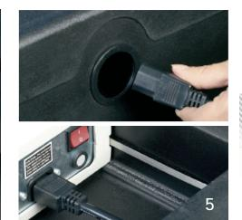
Thread the power cord through the power cord tunnel on the back of the ballot box and connect to the AccuVote unit. Plug the power cord into the UPS unit. Plug the UPS unit into the wall.
