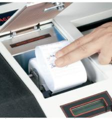
When all necessary reports have printed and been signed, fold or roll at least one report and place it in the printer compartment.
