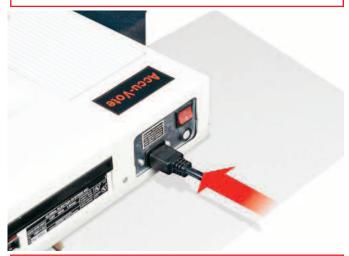
11. Be sure to turn the UPS unit 'On' by pressing and holding the power button until the unit is on.
