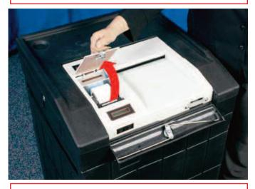
Step 8 – Unlock and remove printer cover
