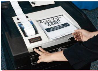
Step 9 – Feed Ender Card while pressing and holding the YES and NO buttons
