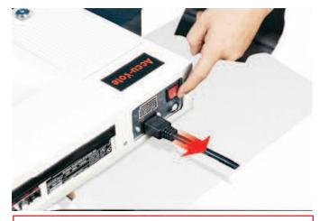
Step 15 – Turn the Optical Scan unit off
