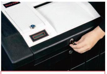
Step 1 – Unlock and open retaining door
