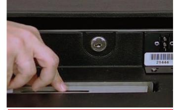
Step 7 – Set the security plate in the groove in the ballot box as shown
