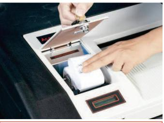
Step 17 – Fold up third copy of tape and replace printer cover
