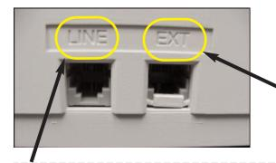
Connect the Inbound / Regular telephone line from the wall to the "LINE" slot on the back of the Fax.
