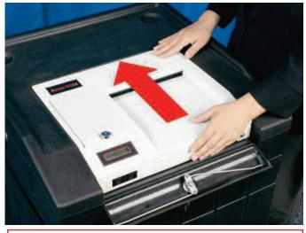
Step 19 – Slide the Optical Scan unit all the way back until securely seated
