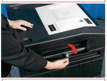
Step 21 – Unlock and open Auxiliary Slot
