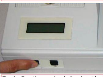
Step 4 – Override overvote rejections by holding the YES button and feeding the ballot
