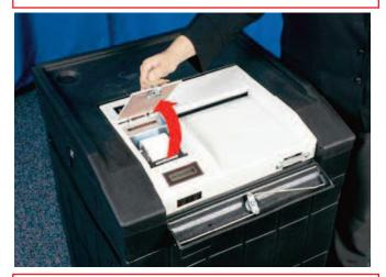
Step 12 – Unlock and remove printer cover.
