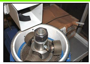
LEFT: Part of a hop-pelletizing machine displayed last week at the annual meeting of the Connecticut Hop Growers Association. Hops ground by hammer mills are brought by augur through a chute (at top of photo) where three metal wheels press the material though small die holes at bottom, forming the pellets.
