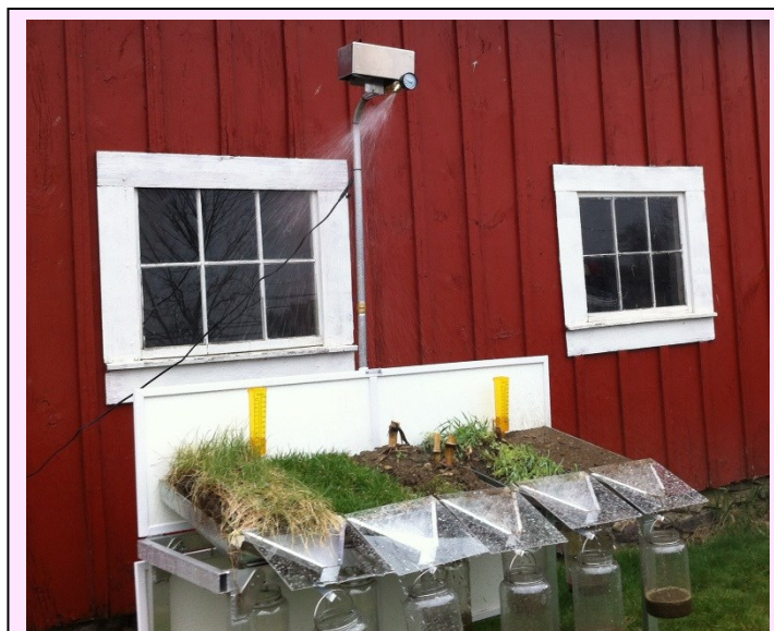
This NRCS rainfall simulator demonstrates water runoff and penetration in relation to crop management using traditional till, conservation till, and no till.
