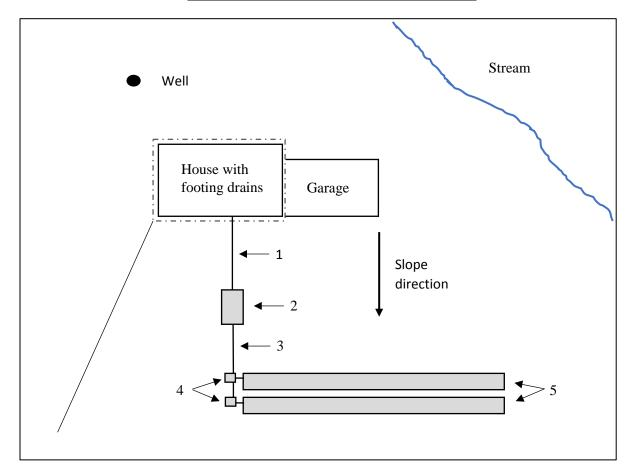
Label the five different septic system components shown in the picture above:
