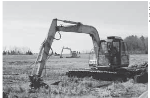
The WHAMM Program's low ground pressure (less than 2 lbs. per square inch) excavators can work in soft, marsh soils to create ponds and plug old ditches.
