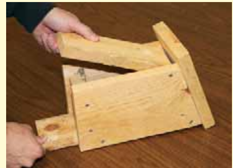
Place the screws near the top of the front piece and directly across from each other so that the front piece can swivel upwards for inspecting the nest.
