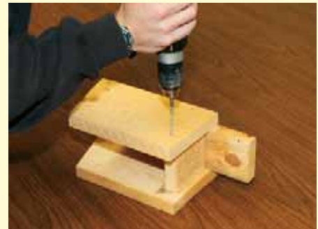
Insert and attach the floor piece approximately 1/2-inch above the bottom of the sides. Use two screws on each side and one in the back.
