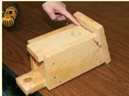
Make sure the front piece fits properly between the two sides. Leave a gap near the top of the front piece. Attach the front piece using two screws.
