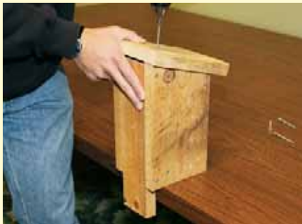
Attach the roof piece using at least four screws. Make sure the roof is set far enough back to prevent rain from entering the vent.
