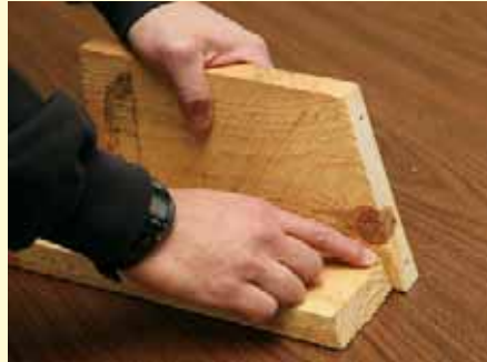
Place one of the sides along the back piece. Be sure to leave a small gap at the top.
