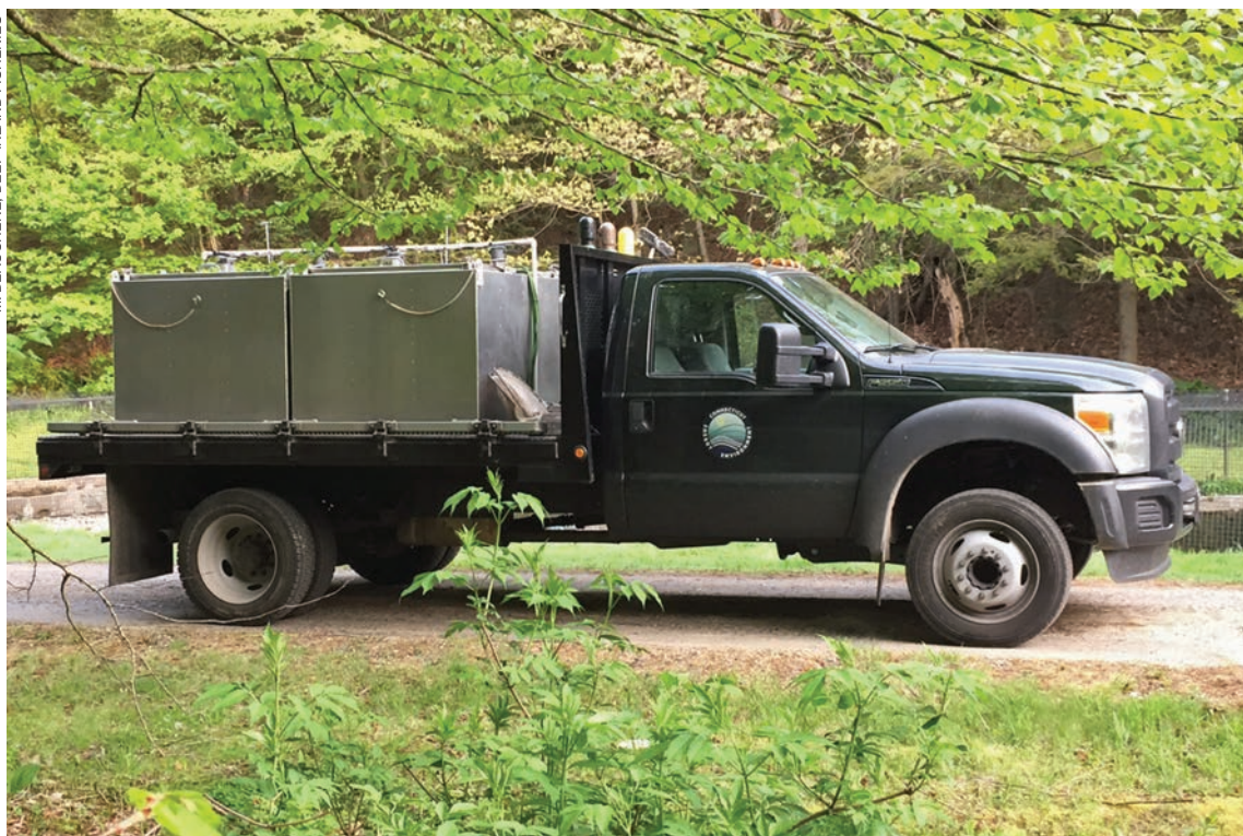
Today, over 600,000 catchable-sized trout are transported to over 200 rivers and streams and 100 lakes and ponds using slightly more “horsepower.” This truck is capable of transporting about 3,000 pounds of fish at a time while constantly aerating the tanks with oxygen.
