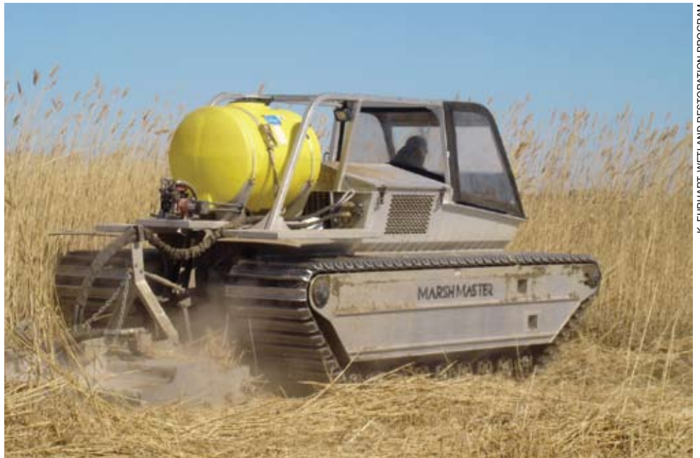
A Marsh Master (an amphibious tracked machine) was used at the Roger Tory Peterson Wildlife Area in Old Lyme to apply herbicide to invasive phragmites and then mow the dead stems.
