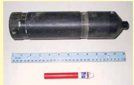
Vemco VR2W acoustic receiver and long-lived ultrasonic transmitter.
