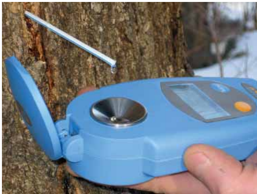
A refractometer is used to measure sap sugar content. Some trees are consistently sweeter than others and should be favored as crop trees.
