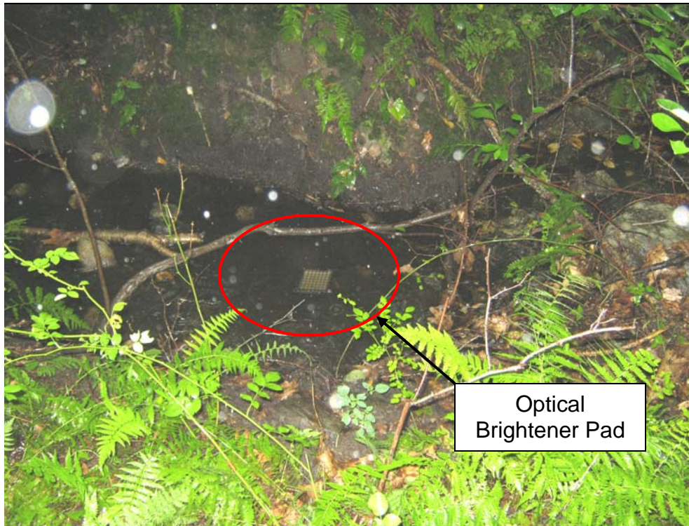
Figure 4: Optical brightener pad in stream north of Ox Hill Road culvert.
