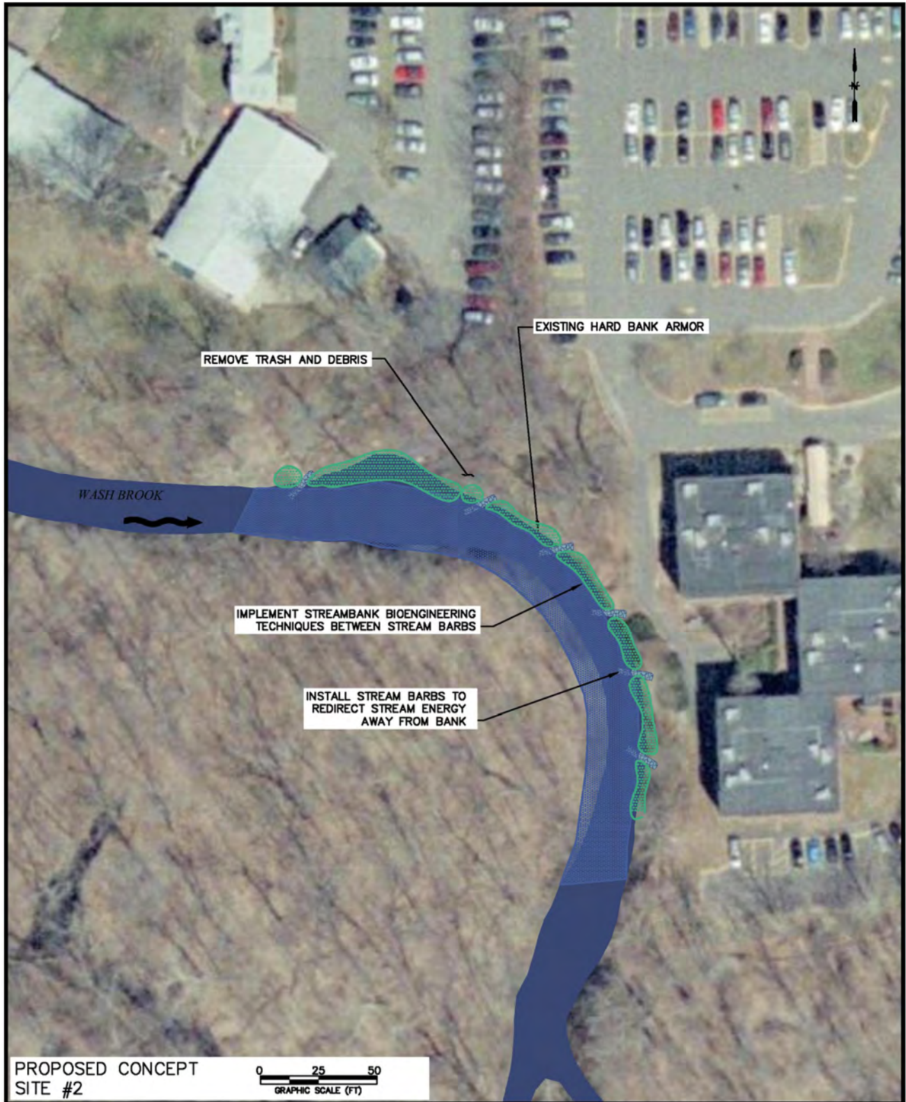
Figure 3-13d. Wash Brook Bank Erosion Site #2 Bank Stabilization Concept
