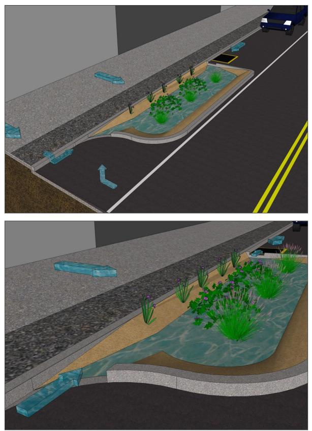
Figure 11: Street-side bioretention bump-out
