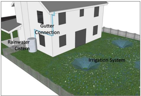
Figure 15: Rainwater harvesting cistern installed behind a house
