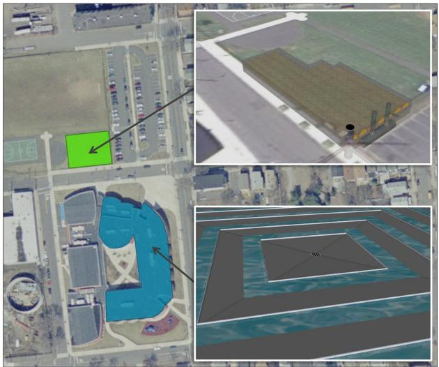
**Figure 9:** Subsurface rainwater harvesting storage (top) and blue roof check dam system (bottom)
