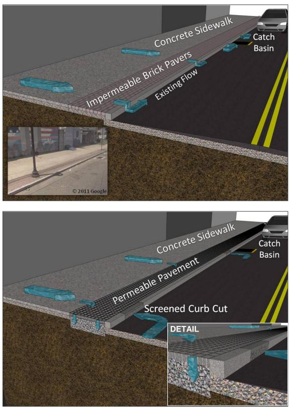
**Figure 18:** Existing sidewalk configuration (top) and proposed permeable pavement retrofit (bottom)
