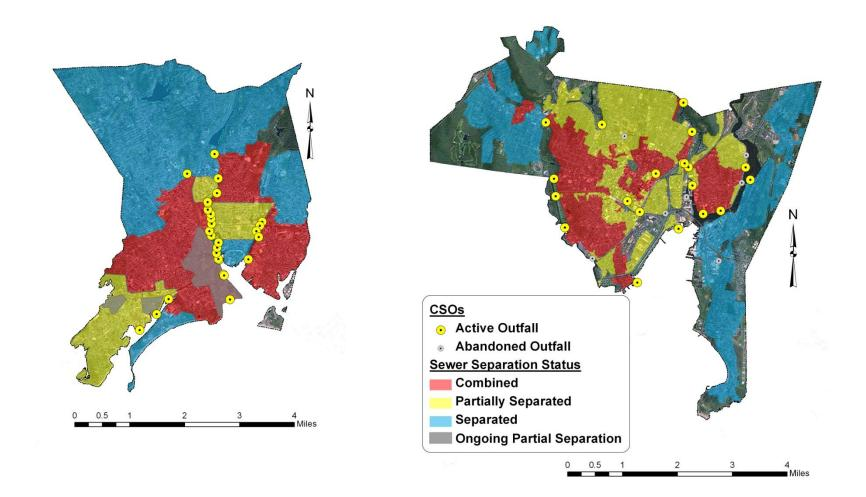
Figure 1: Approximate regions of combined, separated, and partially separated sewers in Bridgeport (left) and New Haven (right)
