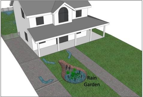
**Figure 16:** Rain garden constructed on a front yard capturing runoff from the rooftop, driveway, and sidewalk
