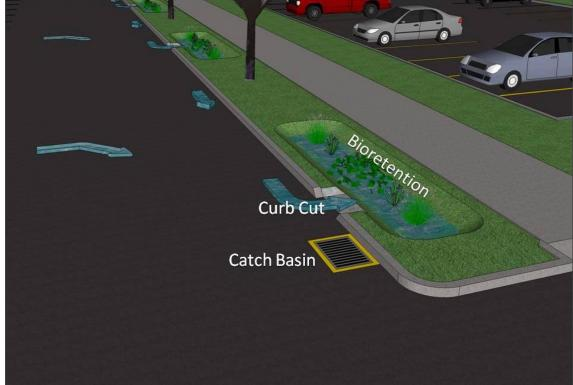
**Figure 8:** Existing parking lot configuration (top) and proposed bioretention concept within parking lot median (bottom).
