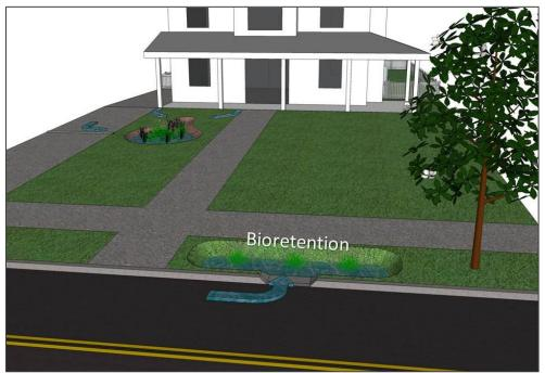
Figure 17: Street-side bioretention capturing runoff from the yard, sidewalk, driveway, and street
