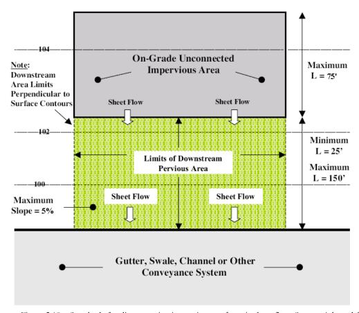
Figure 5.18 – Standards for disconnecting impervious surface via sheet flow. Source: Adapted from New Jersey Department of Environmental Protection, 2004.
