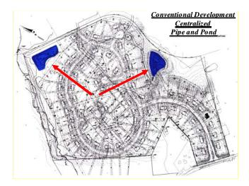
Figure 3.1 – Conventional Controls. A conventional approach requires clear cutting, mass grading and use impervious surfaces, gutters pipes and ponds to collect and treat runoff. This approach completely alters and destroys the natural hydrology and ability of the landscape to absorb rainwater and capture pollutants.
