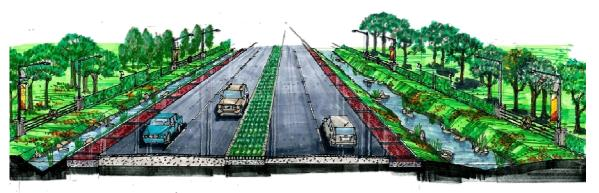
Figure 4.9 - Shoulder Treatment Systems using detention and filtration design.
