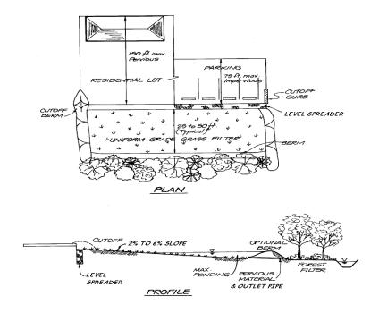
Figure 5.21 – Drawing of a vegetative filter strip. Source: Adapted from Atlanta Regional Commission, 2001.
