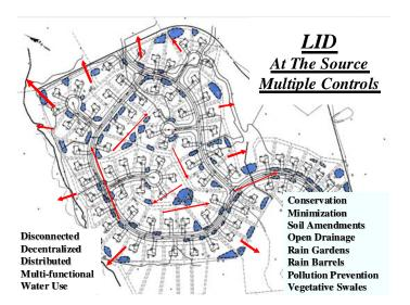
Figure 3.2 – LID Controls. A LID approach use a wide array of techniques that work with the landscape, soils, drainage patterns and vegetation to minimize impacts and integrated management controls to retain, detain, infiltrate and filter runoff. LID can provide better stormwater controls by mimicking the predevelopment hydrology. Often LID designs increase lot yield and reduce infrastructure cost.
