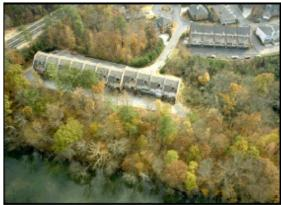
Figure 5.1 - Reduced limits of disturbance minimize water quality impacts. Source: Adapted from Atlanta Regional Commission, 2001.
