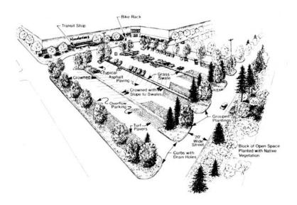
Figure 5.16 – Parking lot with islands attractively integrated. Source: Adapted from Connecticut, 2004.
