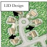
Figure 3.6 - conventional approach of draining runoff to the streets vs. a LID design using site fingerprinting.
