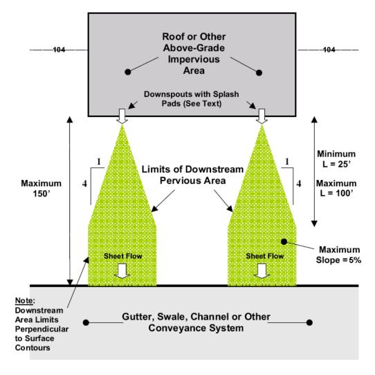
Figure 5.19 – Standards for disconnecting impervious surface via downspouts. Source: Adapted from New Jersey Department of Environmental Protection, 2004.
