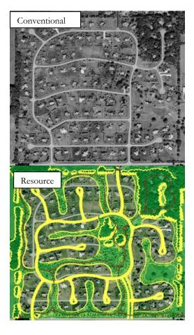
Figure 3.4 – integration of resource conservation into a conventional design.
