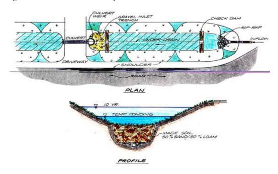
Figure 4.6 - Swale design to enhance its ability to filter and infiltrate runoff.
