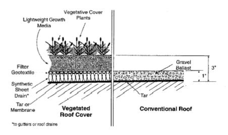
Figure 5.25 – Example Vegetated Rooftop Cross-section
