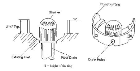
Figure 5.24 - Roof ponding rings. Source: Adapted from Tourbier, 1974.
