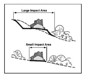
Figure 5.6 – Building on flatter slopes reduces the impact of development. Source: Adapted from Atlanta Regional Commission, 2001.
