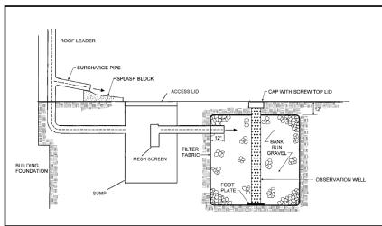
Figure 5.27 – Schematic of a drywell with optional sump to facilitate cleanout. Source: Adapted from New York, 2001.
