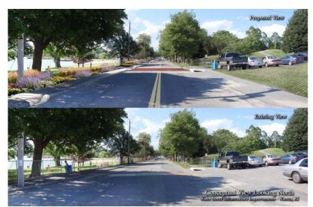
Figure 4.11 – Rain Gardens, Porous Paving Infiltration Chambers in a thickly settled Historic neighborhood and Water front park.
