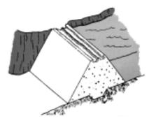
Allows standing water to collect and saturate crest of dam. Vehicles can get stuck. Regrade and recompact crest to provide proper drainage to upstream slope. Install gravel or road base material to accommodate traffic.
