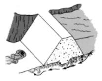
Continuous flows can lead to piping erosion of the foundation and failure of the dam.
