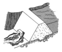
Continued flows can lead to rapid erosion of embankment materials and failure of the dam.
