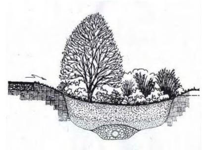
Figure 2.14. Filtration/partial recharge facility
