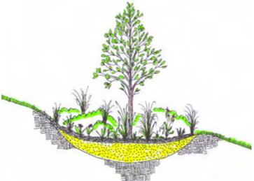
Figure 2.9. Shallow dish (scalloped) bioretention
