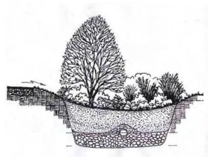
Figure 2.15. Infiltration/filtration/recharge
