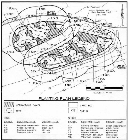
Figure 5.1. A typical bioretention landscape plan
