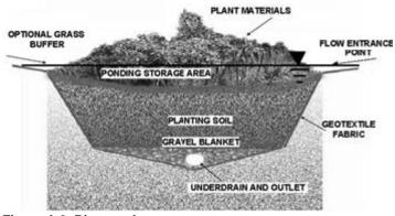
Figure A.3. Bioretention components
