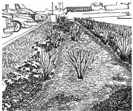
Figure 2.1. Curbless perimeter bioretention
