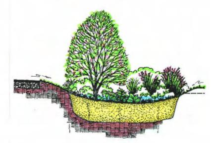
Figure 2.13. Infiltration/recharge facility (enhanced infiltration)
