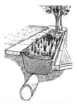
Figure 2.11. Tree-box area bioretention
