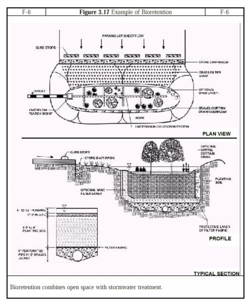
Figure 4.3. Example of bioretention from the state manual
