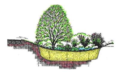
Figure 1.2. Bioretention facility conceptual cross-sectional layout (early design). Impervious area runoff, soil medium consists of sandy material, and early concept relied on infiltration and plant uptake.
