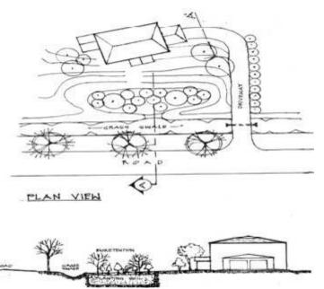
Figure 2.6. Plan view and cross section of a swaleside bioretention area
