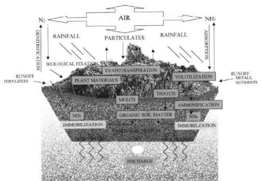
Figure A-1. Nitrogen cycle for bioretention
