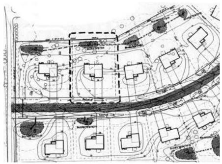
Figure 3.2. Typical site plan with bioretention
