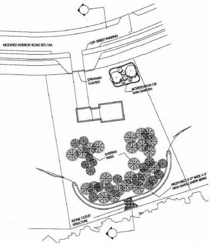
Figure 2.19. Existing wooded area converted with berm
