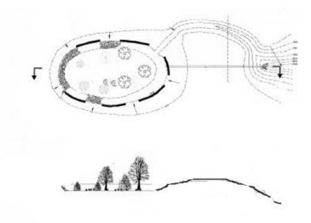
Figure 2.2. Curbless flow-through bioretention
