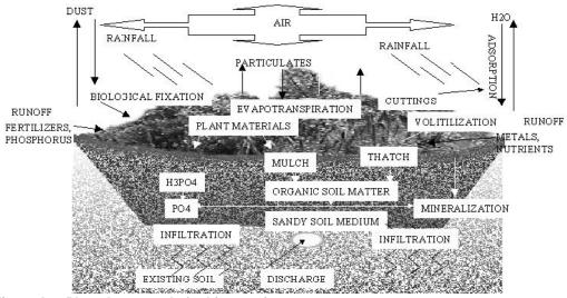
Figure A.2. Phosphorus cycle for bioretention
