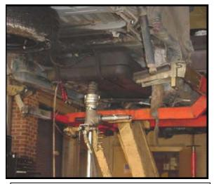
Removing gasoline with a tank drilling machine
