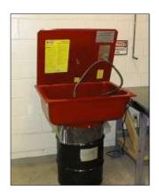
Cold Cleaning Solvent Parts Washer (Lid should be closed when not in use.)
