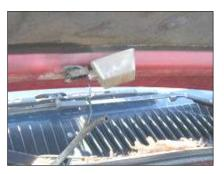
Hood light fixture with mercury switch assembly
