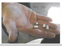
Mercury switches removed from vehicle light assemblies
