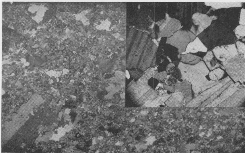
Thin section of "typical" Glastonbury gneiss. Enlargement about 20X. Inset is photomicrograph of encircled area, enlargement 50X.
