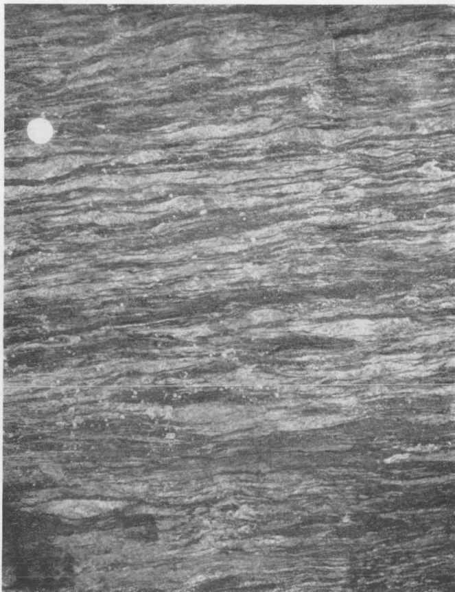
Plate 1, Fig. A. Banded gneiss considered to have developed from mica-quartz schist. Dark bands are mica-garnet-quartz with some kyanite and staurolite. Light bands are quartz and feldspar.
