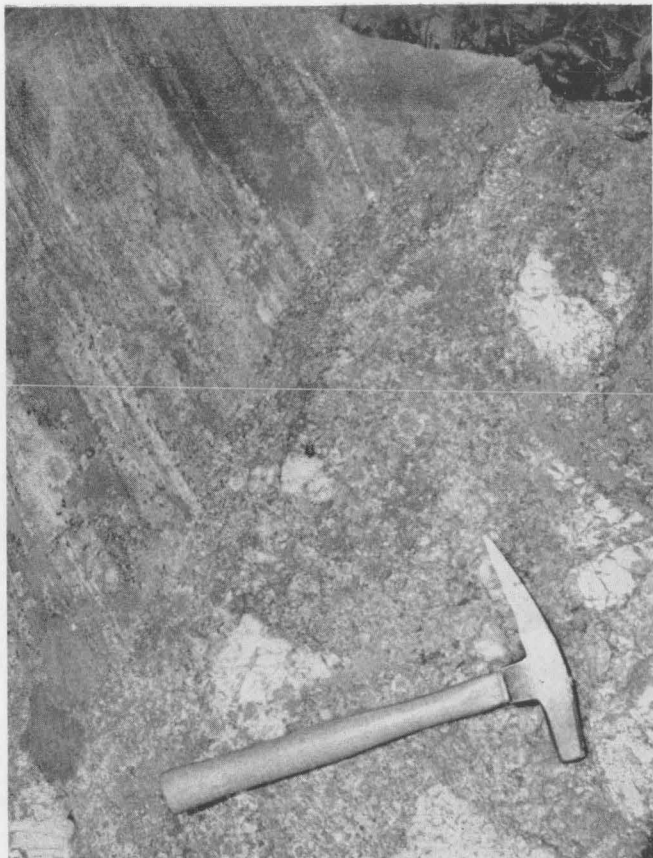
Plate III, Fig. A. Nonewaug granite dike cutting granite gneiss. Notice the fine-grained border and the graphic granite crystals in the granite.
