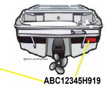
The HIN is typically located on the OUTSIDE of your boat, on the upper right hand corner of the transom. If your boat doesn't have a transom, like a canoe or kayak, then the number will be at the rear of the vessel, on the starboard (right hand) side, near the toprail. If your boat is a pontoon or catamaran, check the back of the starboard pontoon, or aftmost crossmember.
