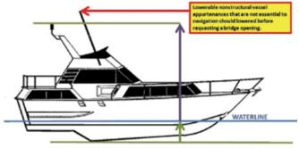
DRAFT = DISTANCE FROM WATERLINE TO LOWEST POINT ON VESSEL
