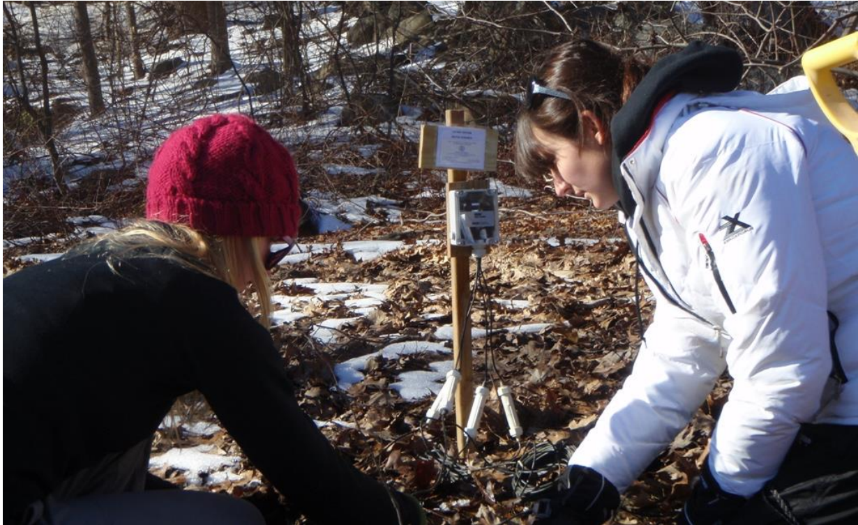
Figure 7. Air and sediment temperature sensors to monitor drawdown conditions (depth 0.6m) in northwest Turtle Cove, January 10, 2013. Note leafy substrate.
