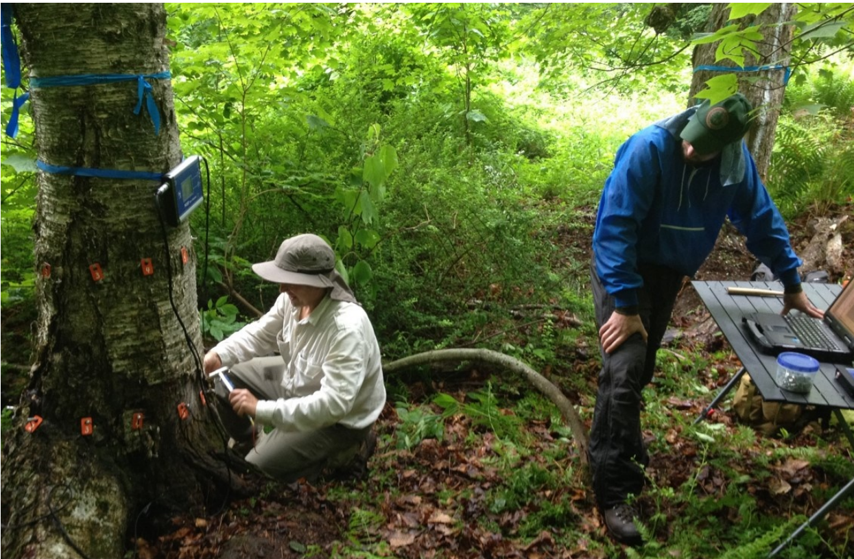
Drs. Marra (left) and Brazee performing a tomographic scan on a yellow birch at Great Mountain Forest.
