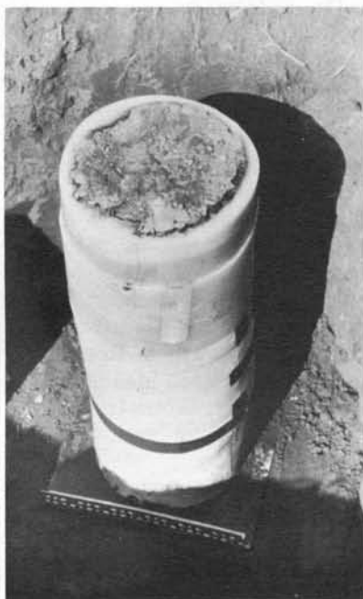
Undisturbed columns of soil, left, were encased in plastic, hoisted out, and taken to the Soils laboratory in New Haven.
