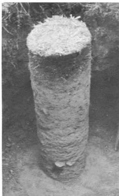
Undisturbed columns of soil, left, were encased in plastic, hoisted out, and taken to the Soils laboratory in New Haven.
