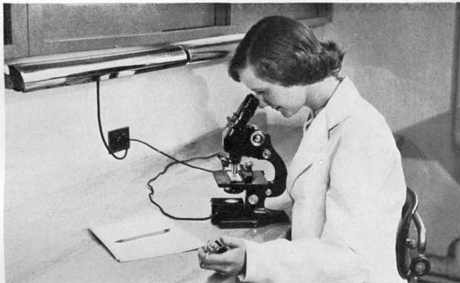
One of the steps in the development of a new fungicide. Slide under the microscope contains a test chemical and spores of a plant disease. Mrs. Elinor Moquette counts the spores to see how many remain alive after overnight exposure to the chemical.
