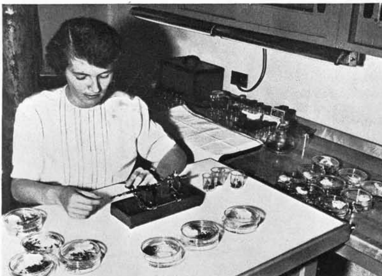
Miss Nancy Woodruff uses a micro-injector to deliver a test chemical directly into the blood stream of a living insect. Basic parts of the instrument are an ordinary hypodermic needle and syringe.
