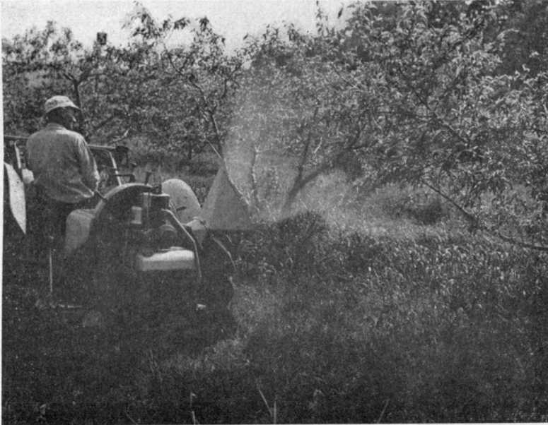
Figure 3. Treating peach trees with the machine mounted 2 feet above the ground so that the fish-tail outlet can deliver spray from a low position.
