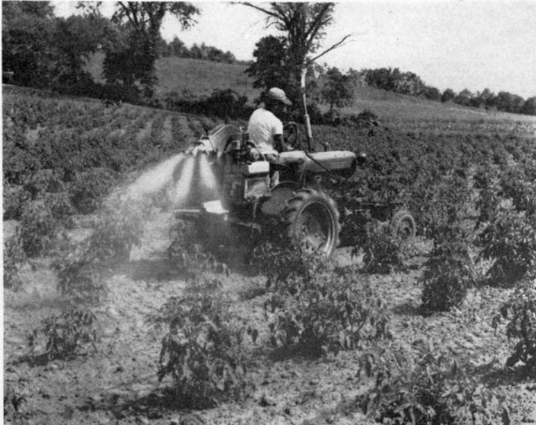
Figure 1. Mist blower mounted on a small tractor with the outlet five feet above the ground for treating row crops. From this position the fish-tail outlet can be used as well as the triple round outlets shown in the figure.
