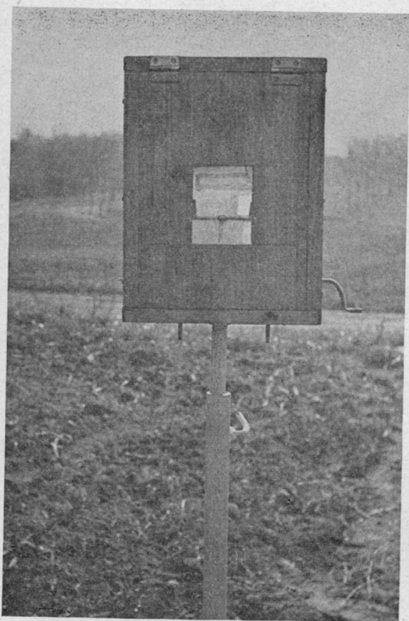
Figure 13. Front view of apparatus shown in Figure 12 in position for taking a particle sample.
