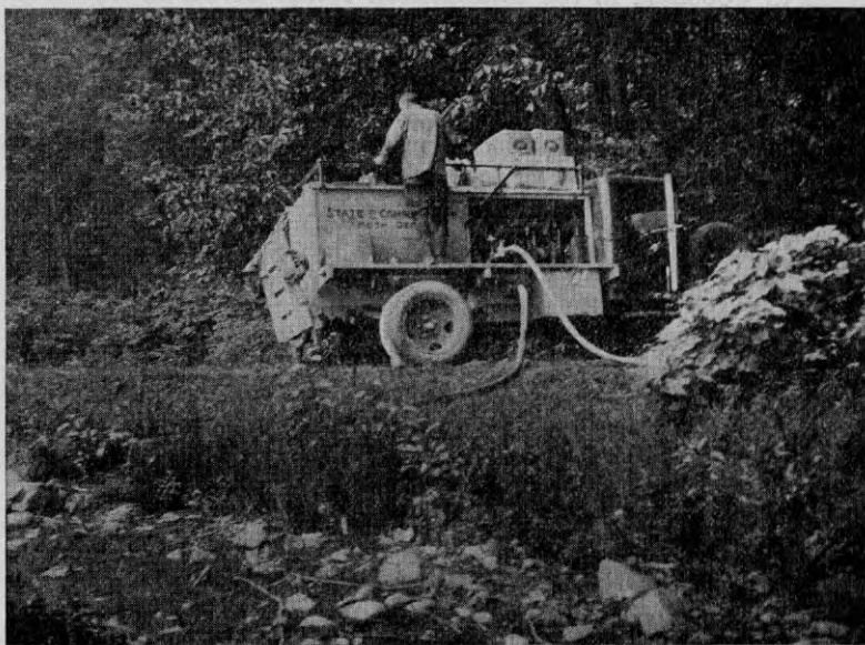
FIGURE 107. New automobile truck power sprayer for gipsy moth work. Photographed in West Hartford, June 21.
