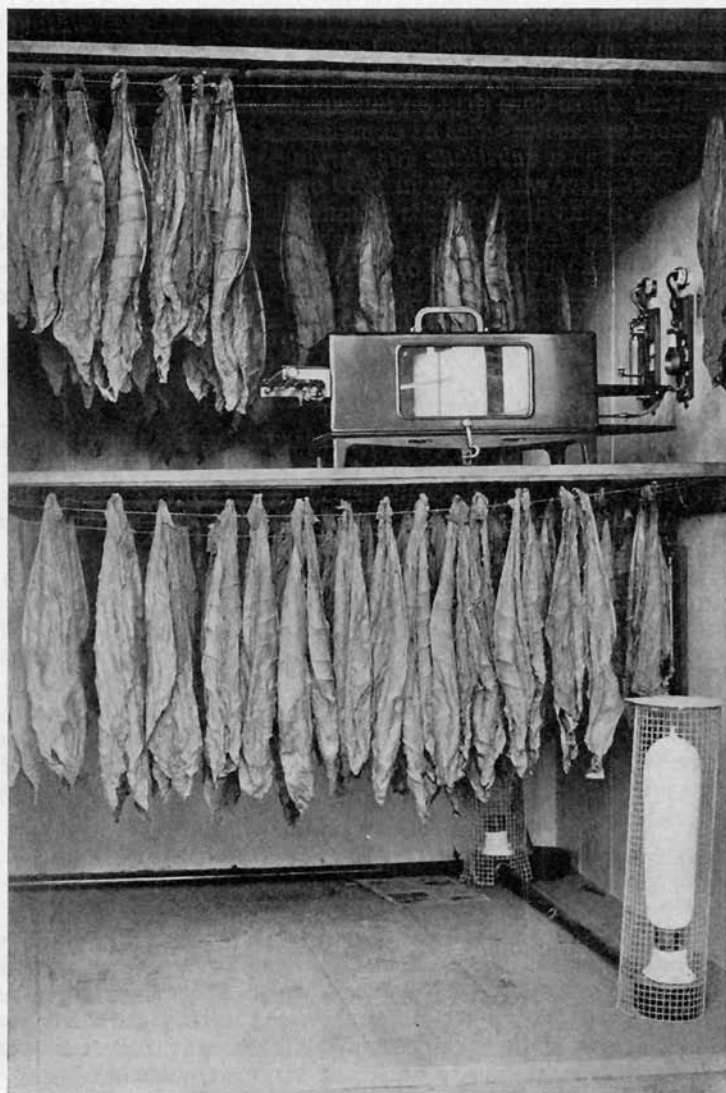
FIGURE 9. Tobacco in the "curing chambers" of the Tobacco Substation, where tobacco is cured in experiments with controlled conditions of temperature and moisture.
