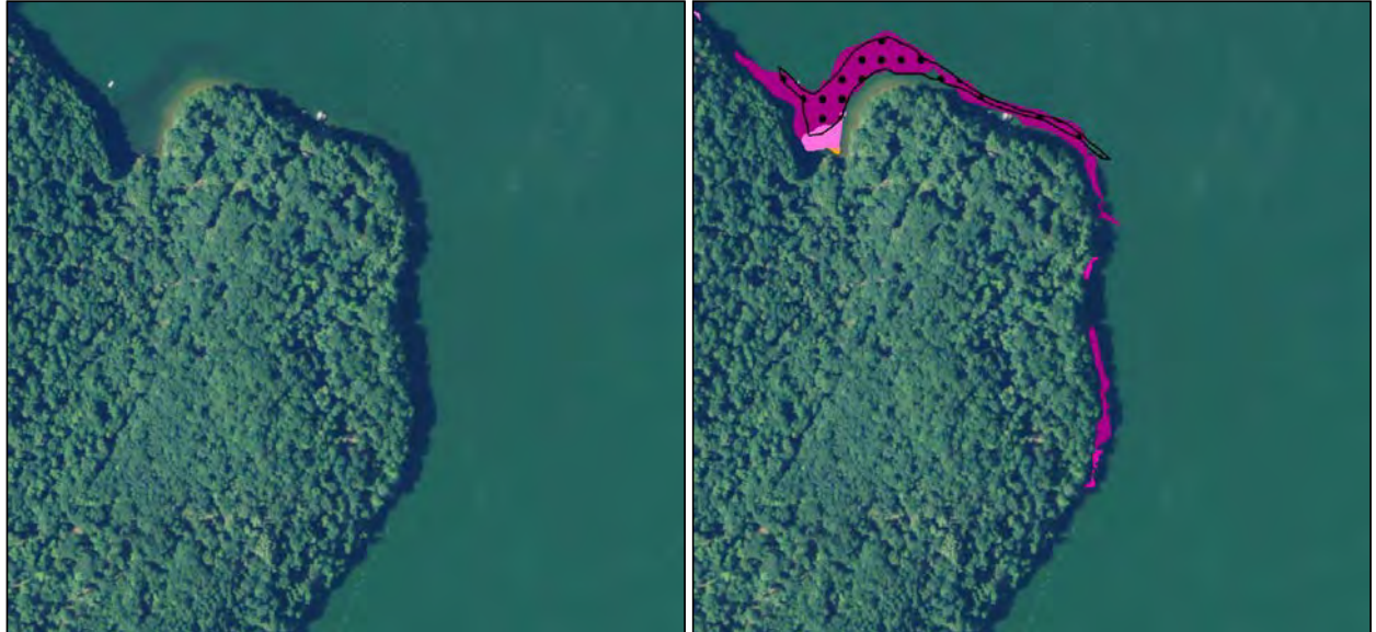
Figure 17. Shadowing from trees or other features along the shoreline (left) can reduce the visibility of plants to remote sensing. Pink and purple shading (right) indicates M. spicatum found by field survey. Dotted areas (right) indicates M. spicatum found by remote sensing
