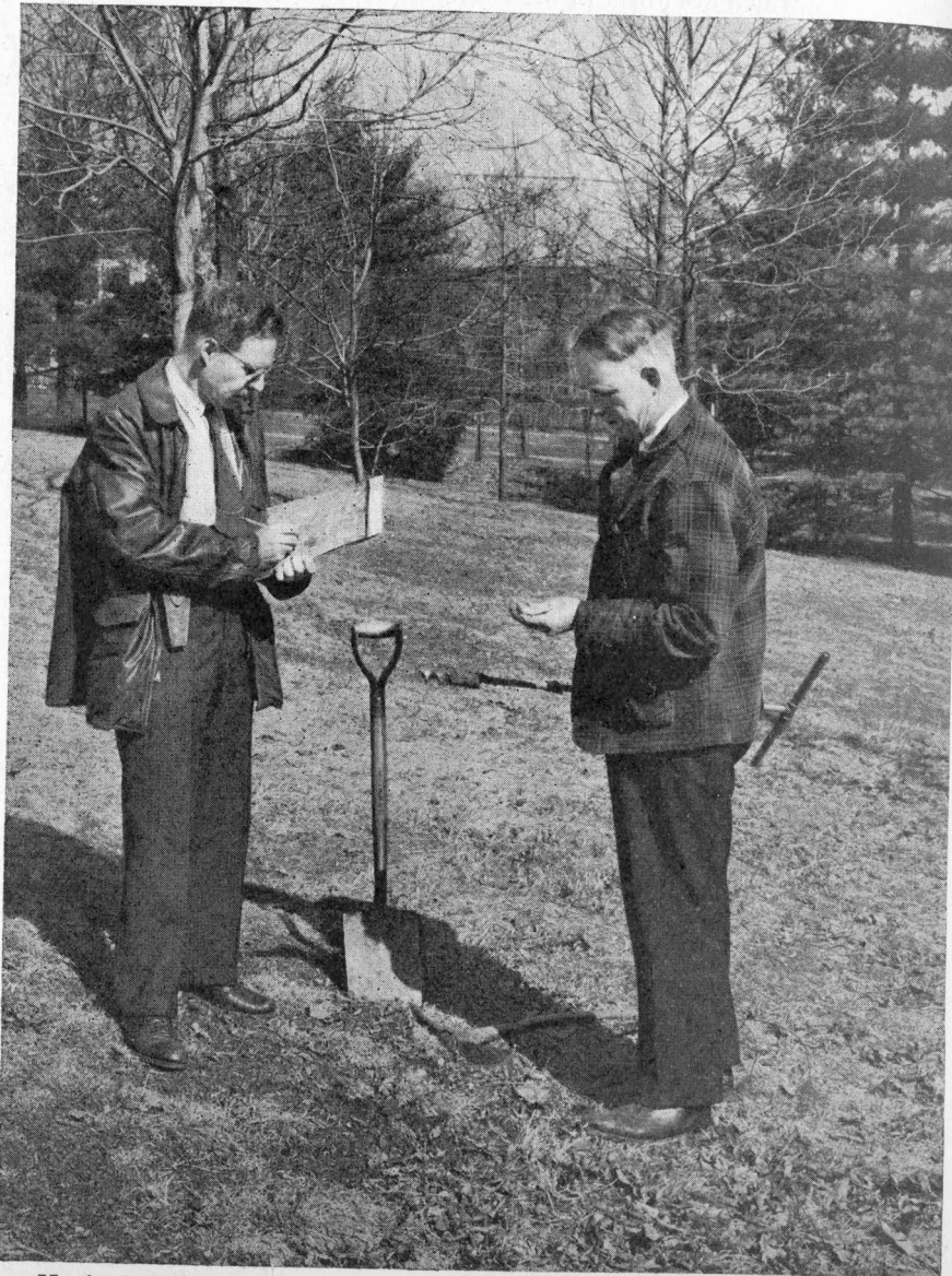
H. A. Lunt and H. G. M. Jacobson surveying soils in the field, the first step in the preparation of soil maps. Mr. Jacobson holds a soil auger which is used to sample soil. Soil, slope, and land use separations are made directly on the aerial photograph which Mr. Lunt holds.
