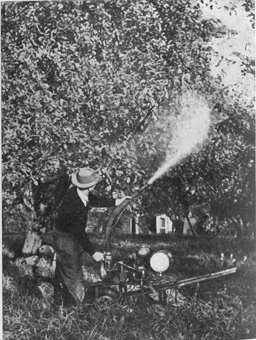
One of the newest methods of applying insecticides is by means of mist blowers. This portable machine, operated here by R. A. Spencer, has a three-gallon capacity and weighs only 86 pounds. It is expected to be useful in nurseries, small orchards, estates, resorts and, possibly, the home garden.
