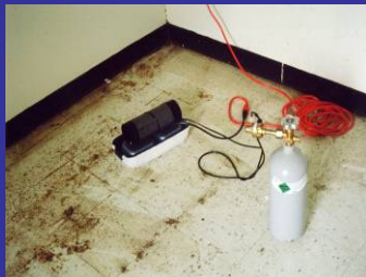
BioSensory trap used to capture bed bugs
