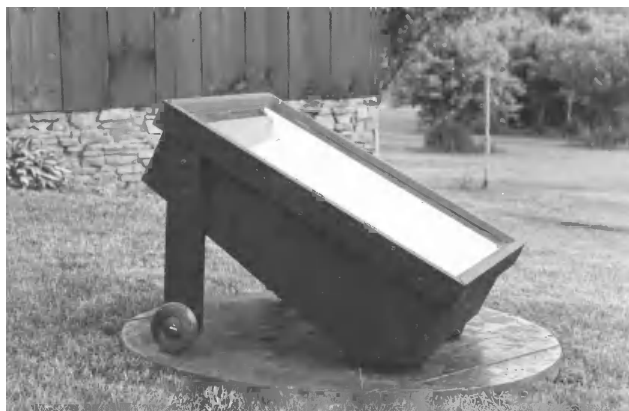
Figure 65. Solar beeswax extractor positioned to receive maximum radiation from the sun and protection from prevailing winds. Placing the extractor on wheels allows it to be moved to face into the sun. (Courtesy of John Harchuck)
