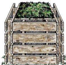
Use 4 pallets to form the sides of the bin and fasten the pallets together with ties. You can also use another pallet for a cover and one more for a base.
