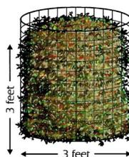
Materials: 14 gauge or medium weight welded wire mesh, heavy-duty plastic ties.
