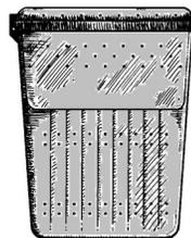
Drill holes all over the sides and bottom of the can. Cover the can to keep animals out of it.
